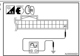
2. Check that signal shown in the figure below can be detected during 10 second just after door lock and unlock switch (driver side) is turned "LOCK" or "UNLOCK".
