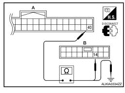
3. Check continuity between BCM connector M18 (A) terminal 40 and ground.
