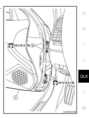
INSTALLATION Installation is in the reverse order of removal. **NOTE:** Adjust the door. Refer to <u>DLK-194, "FRONT DOOR : Adjustment"</u>.
